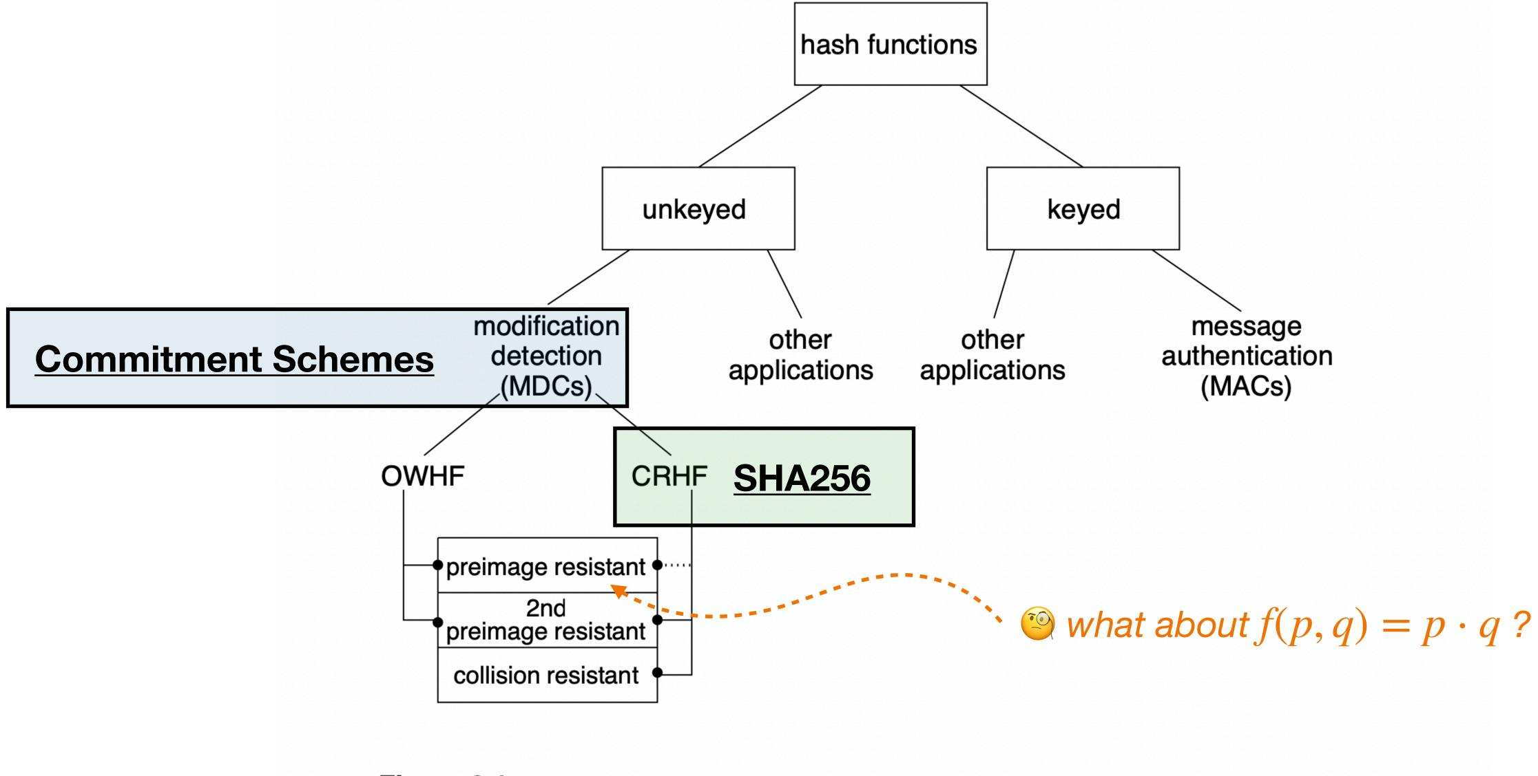
**Figure 9.1:** Simplified classification of cryptographic hash functions and applications.
